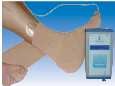
Pressure measurement beneath the elastic stocking and beneath the bandage.
